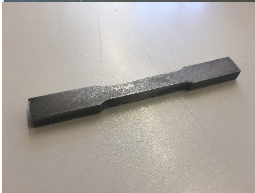
Print of a steel specimen for tensile tests. The specimen is moulded, sintered and finished to machine tools before being subjected to tensile tests.
