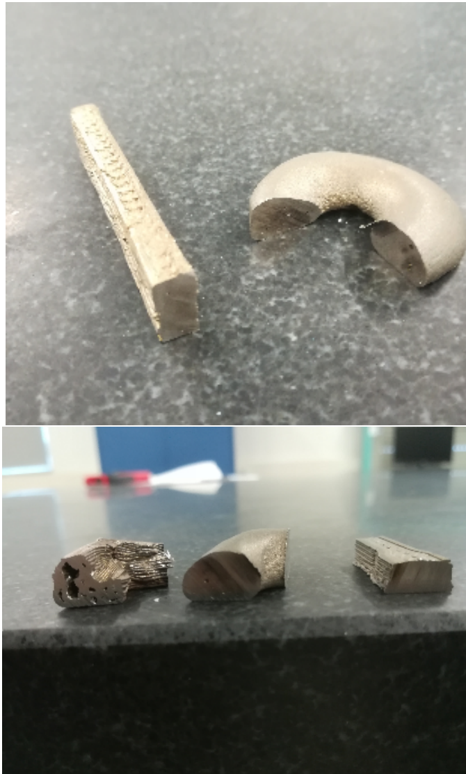
Sintered parts, cut and polished for a study of porosity.
