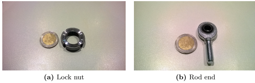
Figure 2.45: Components of the universal joint
