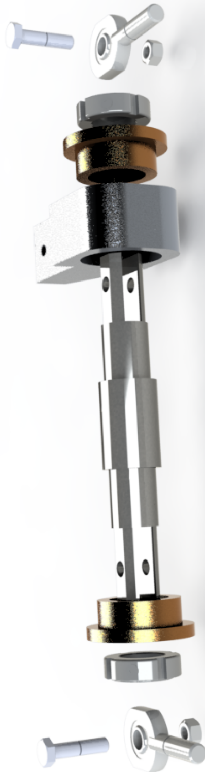
Figure 2.41: Exploded view of the universal joint on the platform
