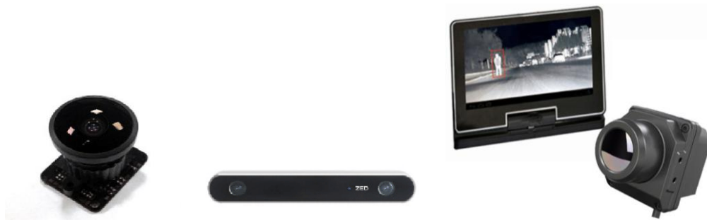
Fig. 3. From left to right, there are monocular camera, stereo camera, and IR camera.
